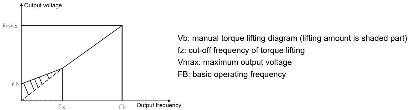
Figure 5 - 04 schematic diagram of manual torque boost
