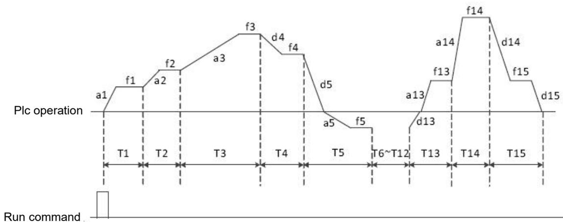
Figure 5 - 33 PLC maintains final value after single cycle
