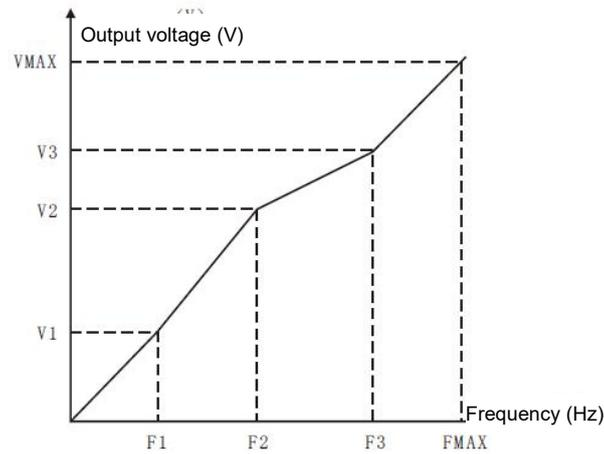
Figure 5 - 05 multi-point V/F curve setting diagram
