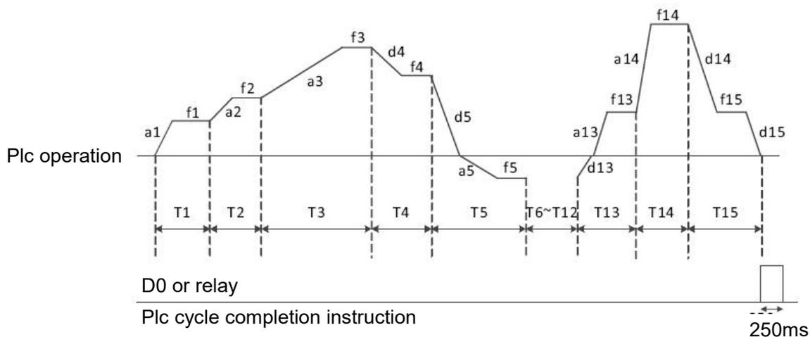
Figure 5 - 31 simple PLC operation diagram
