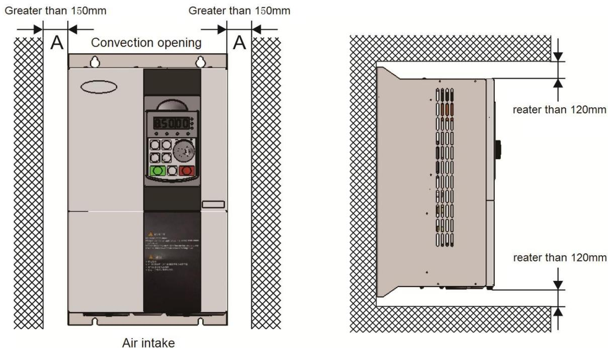
Monomer installation: the size of A is larger than 150 mm, because the upper and lower directions are air ducts, the space distance should be increased.
