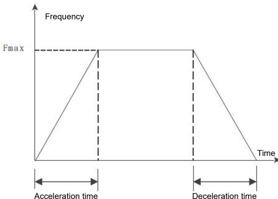
Figure 5 - 20 linear acceleration and deceleration
