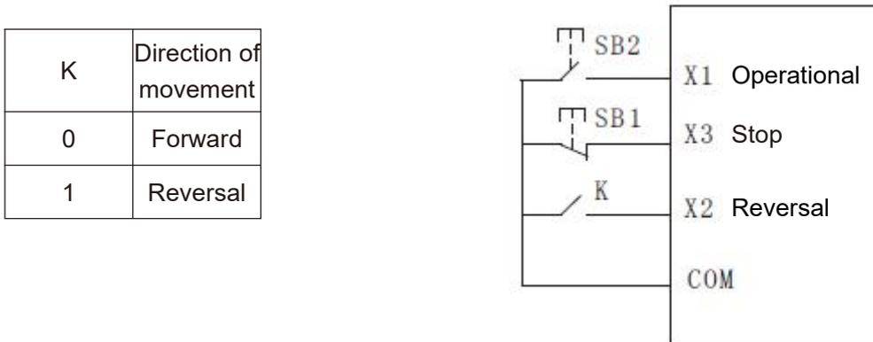
Figure 5 - 15 three-wire control modes 2
