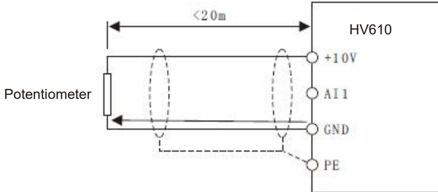
Wiring diagram of analog input terminal
