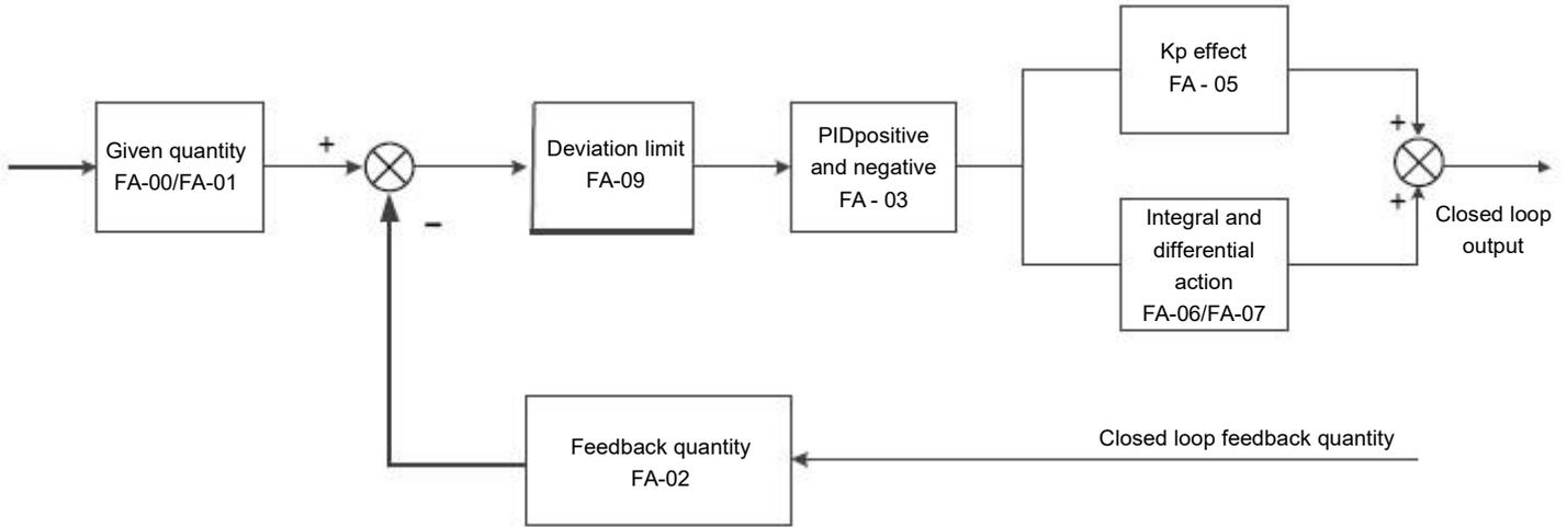
Figure 5 - 27 process PID principle block diagram
