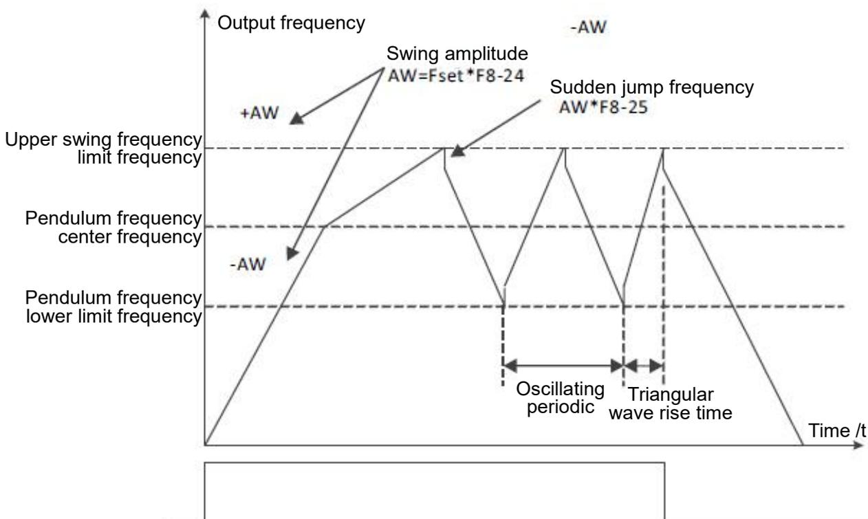
Figure 5 - 24 schematic diagram of swing frequency operation
