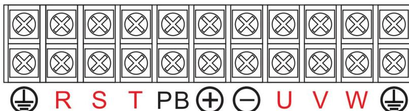
3) Main loop terminal of frequency inverter of 45kw and above:
