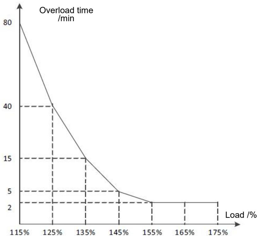
Figure 5 - 25 overload current vs. overload time curve
