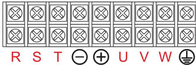
Description of main circuit terminal of three-phase frequency inverter
