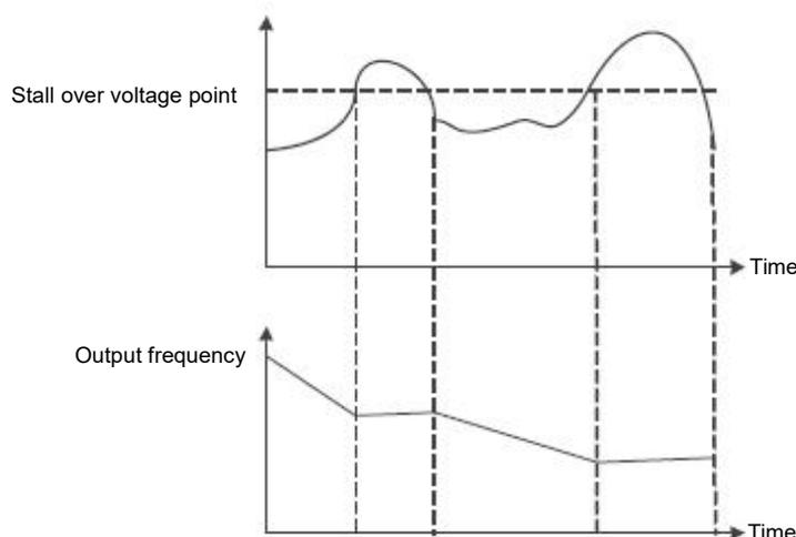
Figure 5 - 26 over voltage stall function
