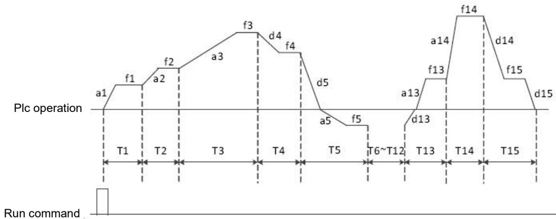
Figure 5 - 32 shutdown modes after single cycle
