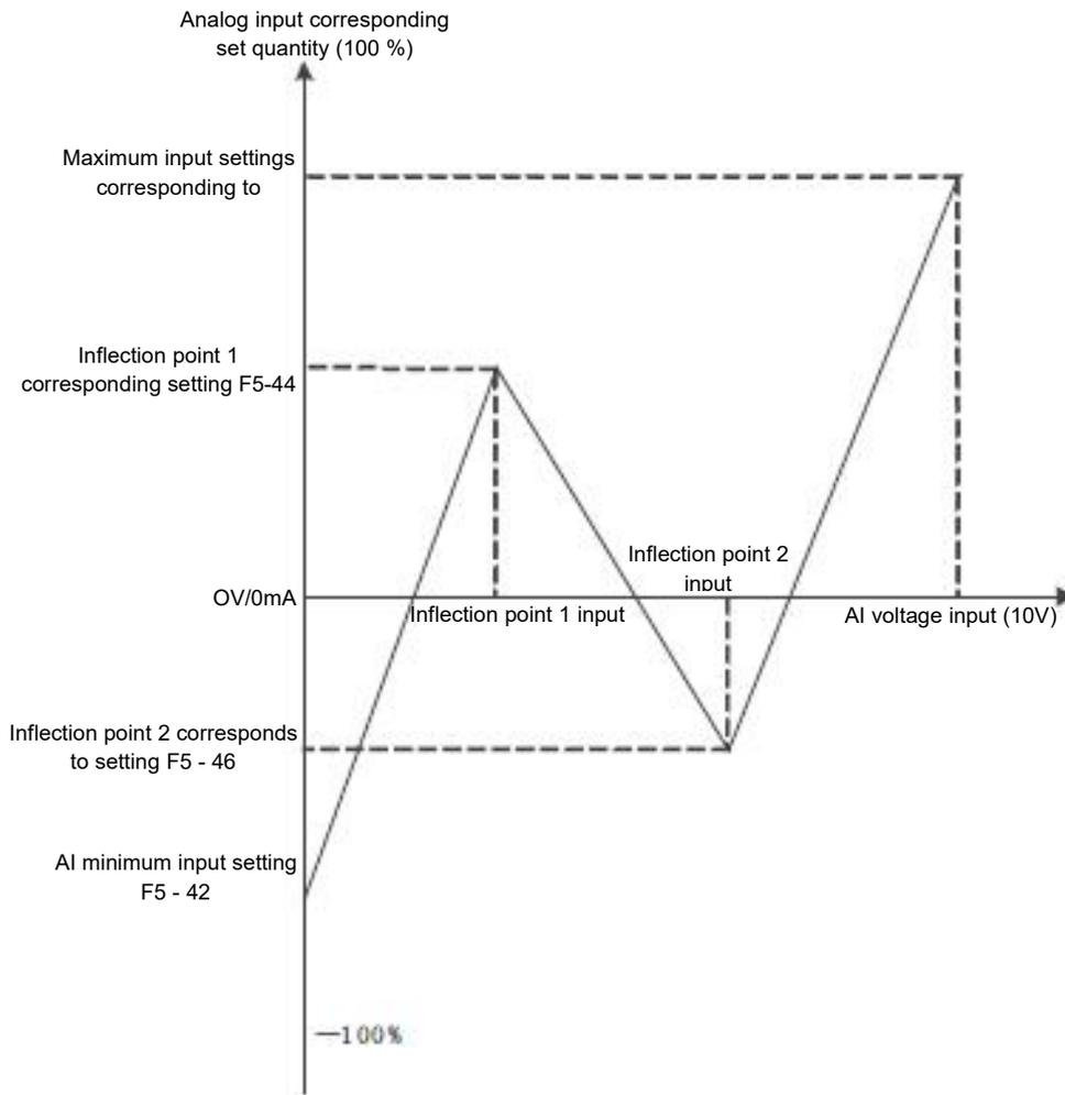
Figure 5 - 17 schematic diagram of 4 - point curve
