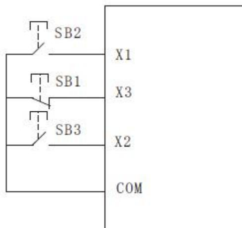
Figure 5 - 14 three-wire control modes 1
