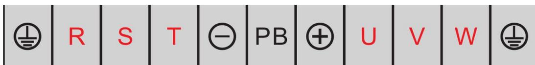
2) 30kw / 37kw frequency inverter main circuit terminal:
