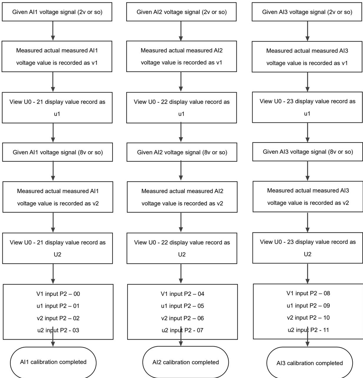
Figure 5 - 34 AI calibration method diagram
