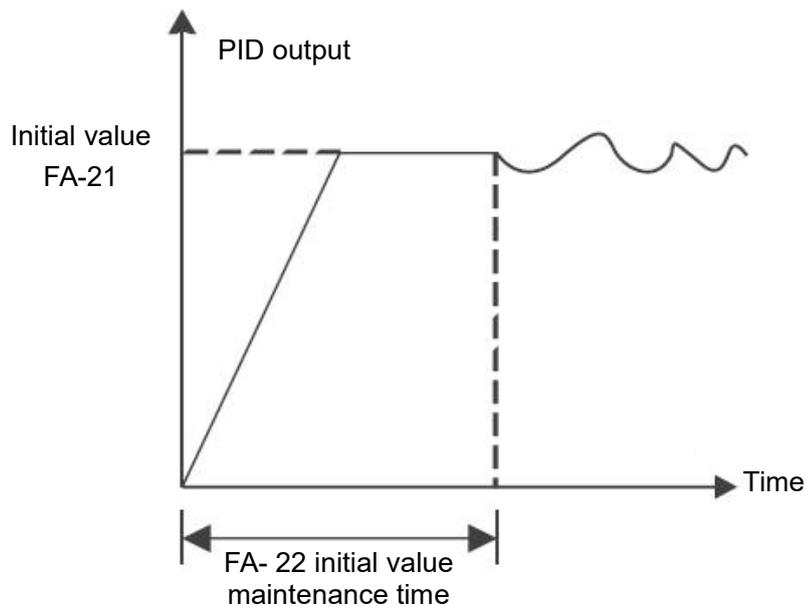
Figure 5 - 30 functional diagram of PID initial value
