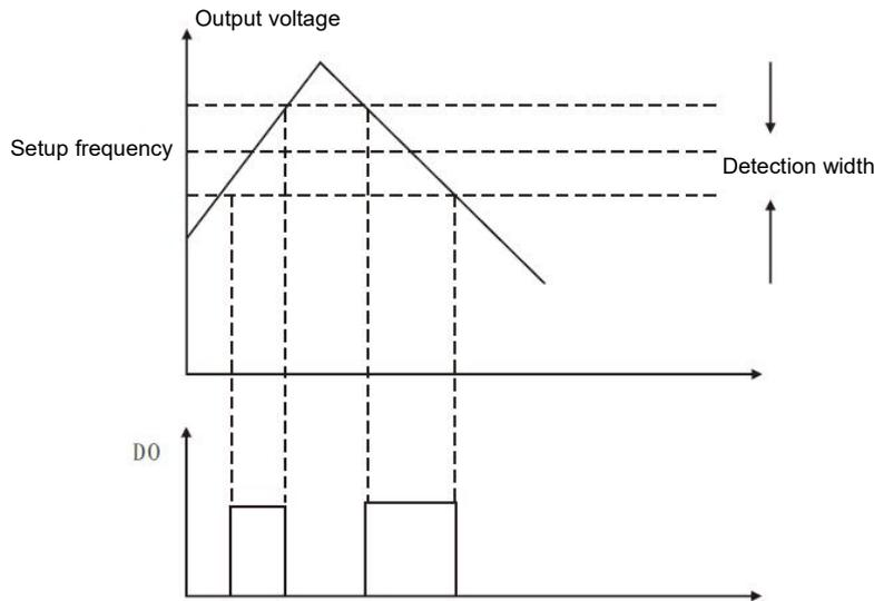
Figure 5 - 10 schematic diagram of frequency arrival detection amplitude
