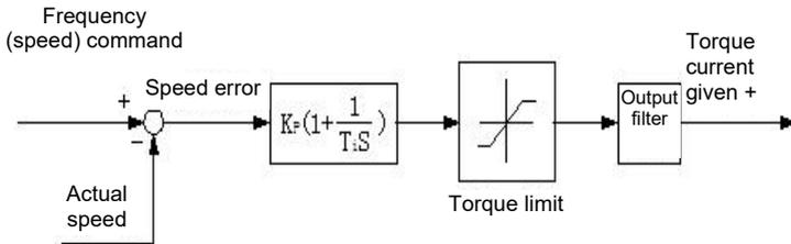
Fig. F4 -1 simplified diagram of speed regulator
