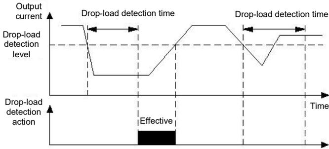
Figure 010-3 Schematic diagram of drop load detection
