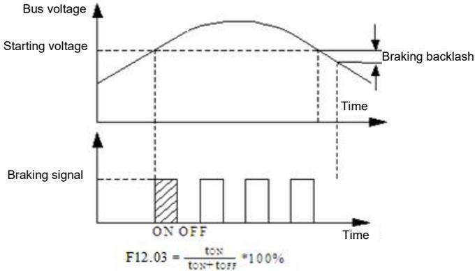
Figure 012-1 Schematic diagram of energy consumption braking
