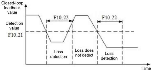
Figure 010-4 Closed-loop feedback loss detection timing diagram
